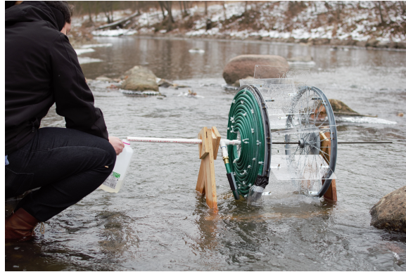
Figure 8: Recording flow rate with finished water pump
