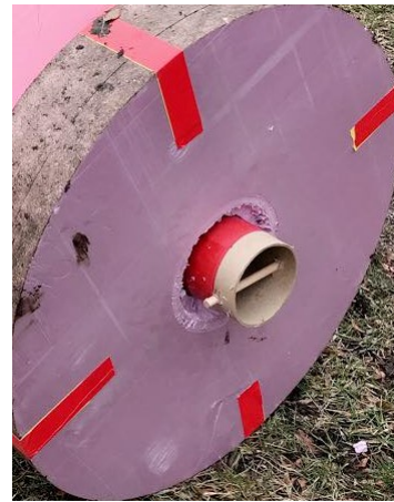
Fig. 26: Securing dowel pin began to tear the wheel apart
