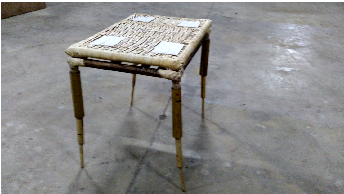
Figure 7.2: Final product ( All legs expanded and table surface oriented horizontally )
